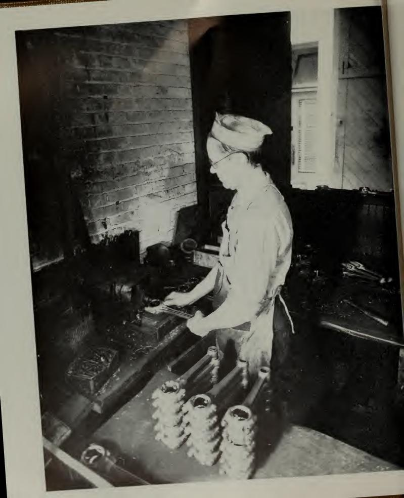
All connecting rod bearings are now given a final inspection and the nuts holding the connecting rod caps in place are loosened to enable the workman to make certain that the bolt or stud threads have not been stripped. The nuts are loosened by a power operated socket wrench as shown in the above picture.
